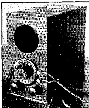
CHECKING THE MODULATION OF THE 'PHONE TRANSMITTER IS JUST ONE OF THE JOBS THAT THIS HOME-MADE NEON-TUBE OSCILLOSCOPE CAN DO
